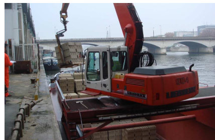
Fig. 37: Ships with own cranes delivering building materials on innercity stocks
