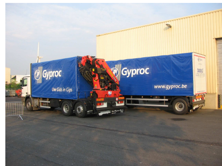
Fig. 32: Gyproc's Python is a combination of a compact truck equipped with crane and a separate trailer
