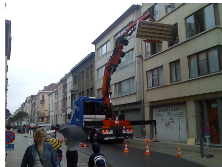
Fig. 32: Gyproc's Python is a combination of a compact truck equipped with crane and a separate trailer
