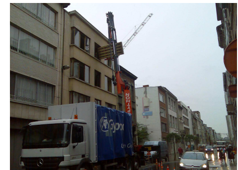
Fig. 32: Gyproc's Python is a combination of a compact truck equipped with crane and a separate trailer
